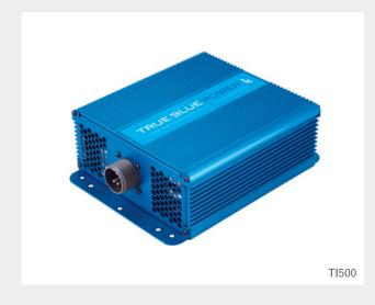
The TI500 DC-to-AC Inverter produces 115 volts at 60 Hz for 500 watts of "wall outlet" power from an aircraft's 28 VDC input. Lighter and 30% smaller than competing inverters, the TI500 has the same connector and footprint of legacy designs, plus overload and short-circuit protection up to 150% of the rated load.
